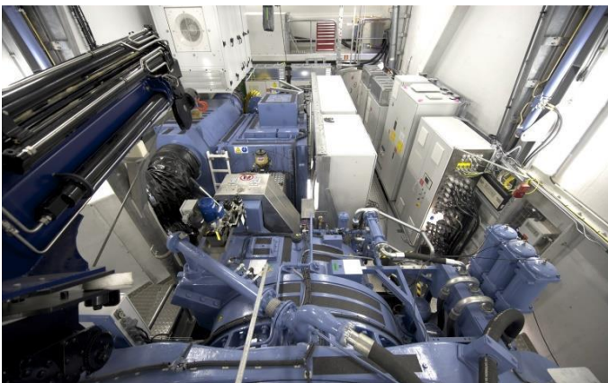
Drivetrain inside the hub of a wind energy system
