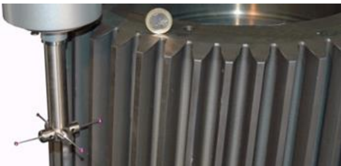
Tactile measurement of large cylindrical gearing
