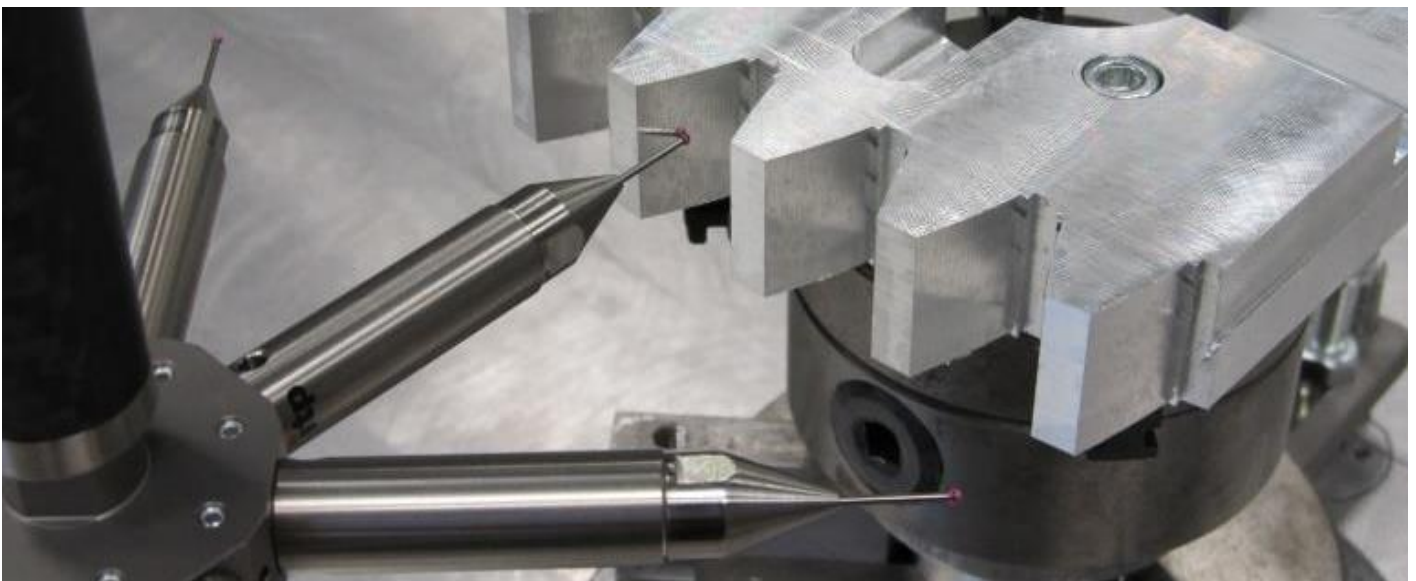
Tactile measurement of a 5-axis milled gear segment
