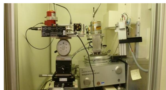
Experimental setup using XRD and photothermal radiometry
