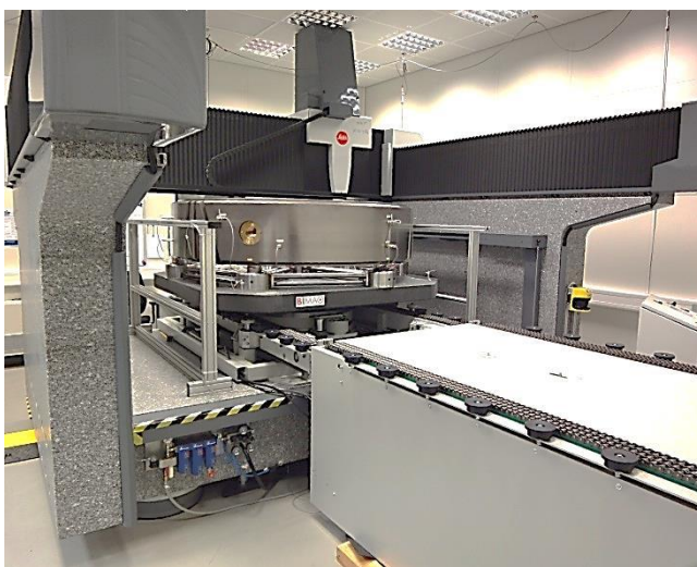
Coordinate measuring machine measuring the large gear standard
