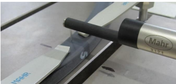
Roughness measurement on a flexible sealing element
