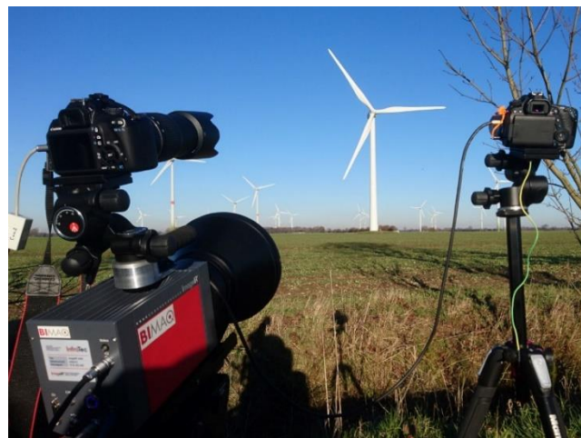
The noncontact temperature measurement from a distance takes place with special cameras and with the help of infrared thermal radiation.
