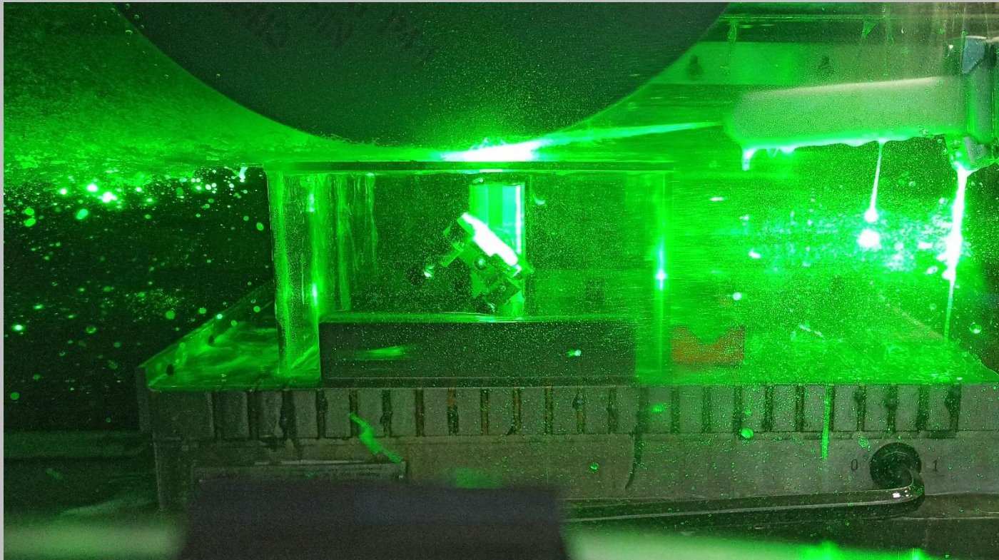
Laser-based measurements of the coolant flow velocity field in a grinding machine
