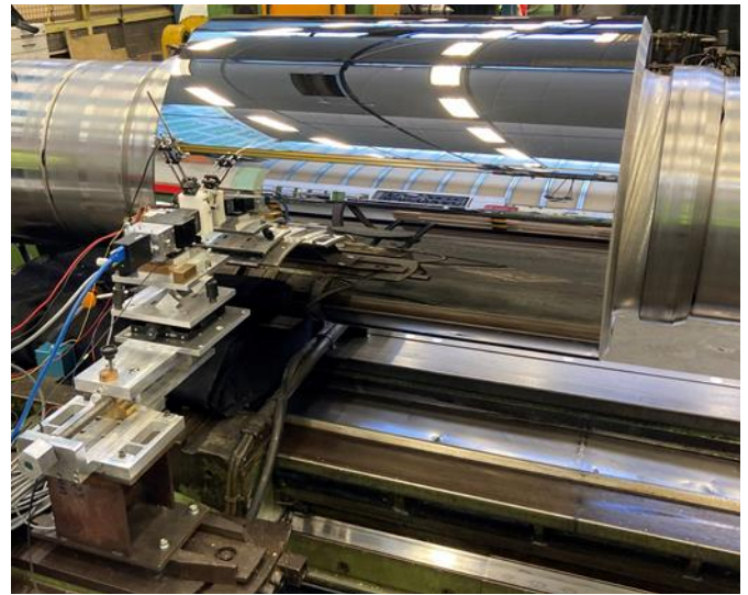
LSWLI setup measuring on a 600 mm roller at Tatasteel's sheet metal plant in Düsseldorf.
