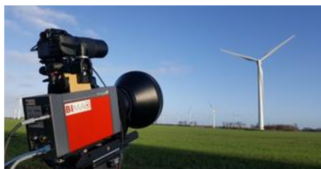
Thermographic flow visualization on wind turbine in operation with an infrared camera
