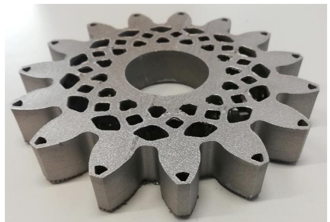
First demonstrator of an additively manufactured lightweight gear. Compared to a solid gear, the weight is reduced by 55 %. Fine machining and experimental load tests are the next steps.
