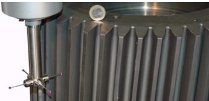
Tactile measurement of large cylindrical gearing
