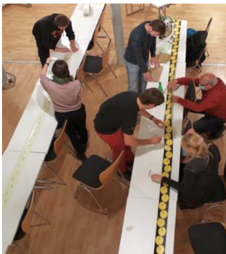
Fig. 1: Fixing the wool threads on an adhesive tape in preparation for tuft assembly.
