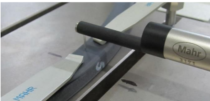
Roughness measurement on a flexible sealing element
