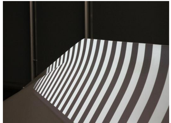
Reference measurement on a blade by means of stripe pattern projection.
