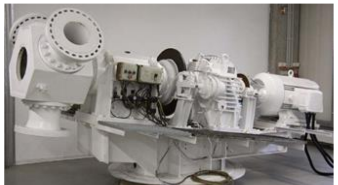
Wind turbine drive train for sensor tests
