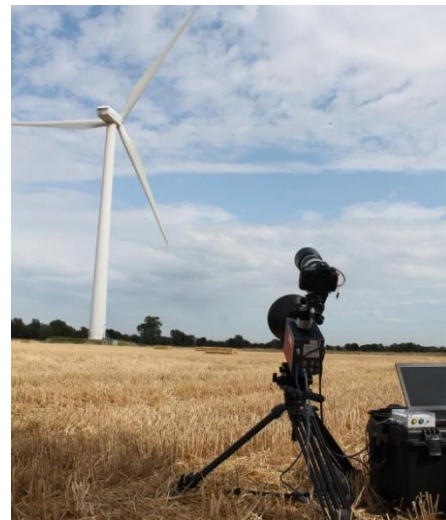
Thermographic flow visualization on a wind turbine in operation with an infrared camera.
