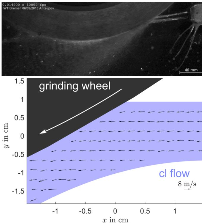
Visualization (top) and PIV measurement (bottom) of the mean cooling lubricant (cl) flow velocity field near the grinding wheel.
