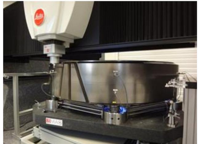
Measuring a 2 m gear standard
