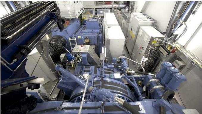
Drivetrain inside the hub of a wind energy system
