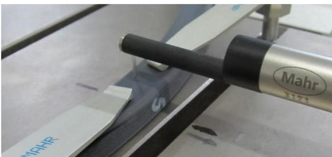
Roughness measurement on a flexible sealing element
