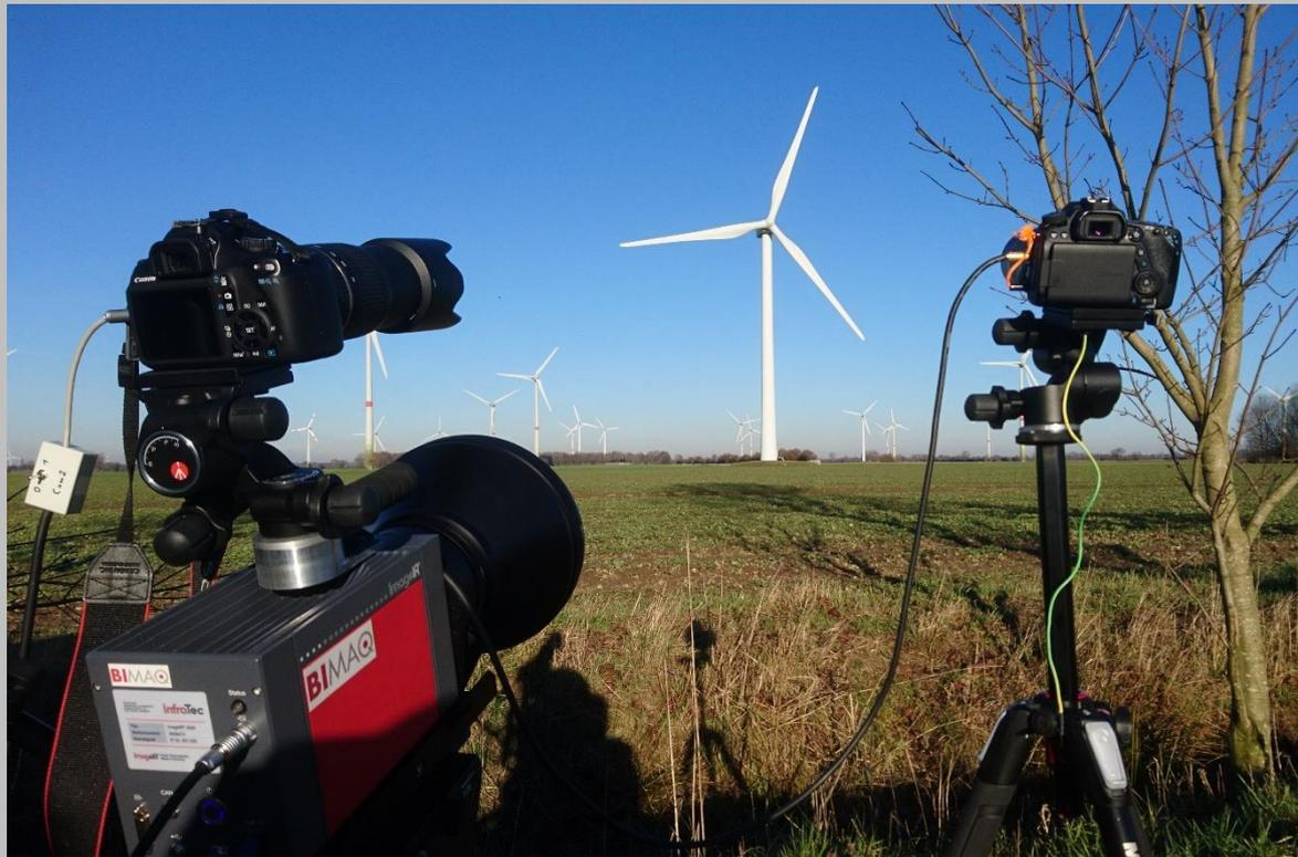
Thermographic flow measurements on wind turbines in operation
