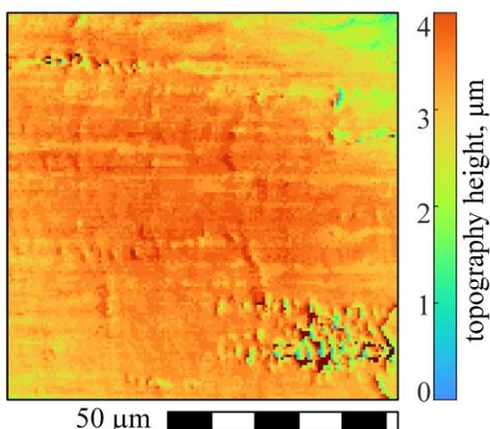
LSWLI topography measurement of a sheet metal strip, mounted on a rotating cylinder with 22.6 mm diameter.
