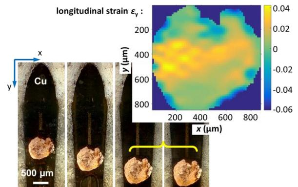
In situ measurements of three steps in the forming history for a Cu micro sample with diameter of 700  $\mu\text{m}$  (bottom left) and the strain  $\epsilon_y$  in the forming y-direction induced in the micro sample after the last forming step (top right).
