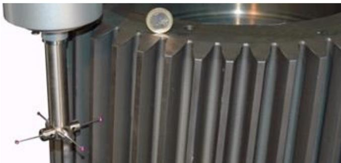
Tactile measurement of large cylindrical gearing
