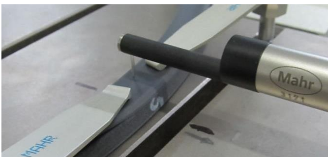
Roughness measurement on a flexible sealing element
