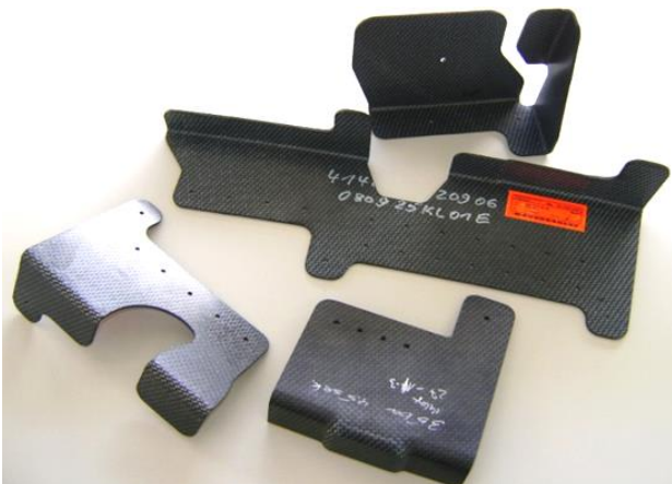
Fiber composite clips of aerospace industry (source: Faserinstitut Bremen e. V.)
