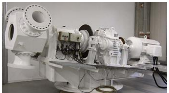
Wind turbine drive train for sensor tests
